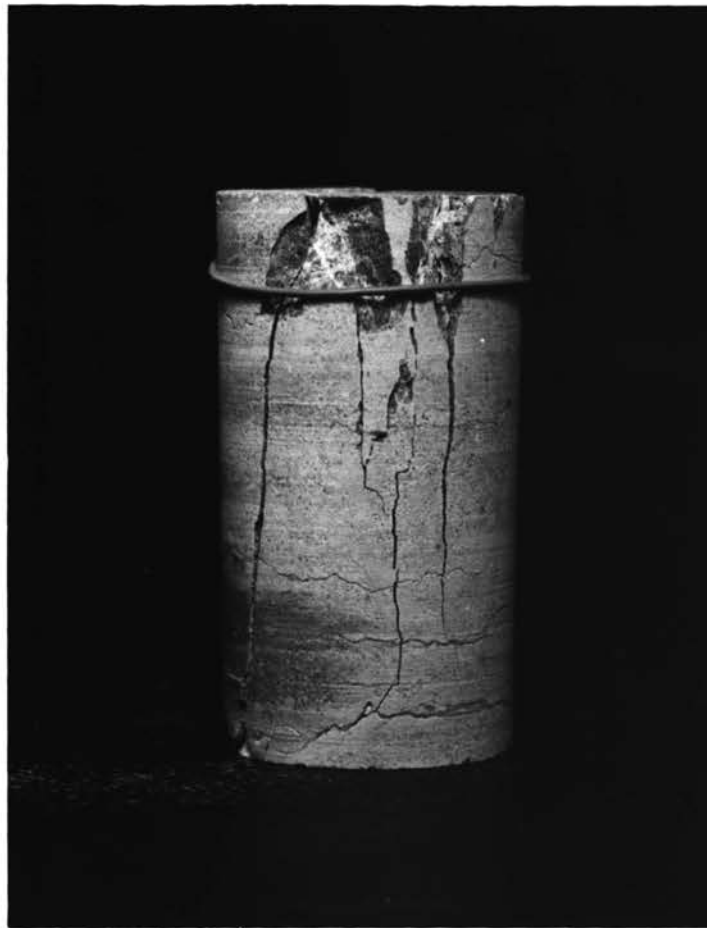
Figure 44 Compressive Failure of a Pea Ridge Dolomite Sample Under a Condition of 3dE.
