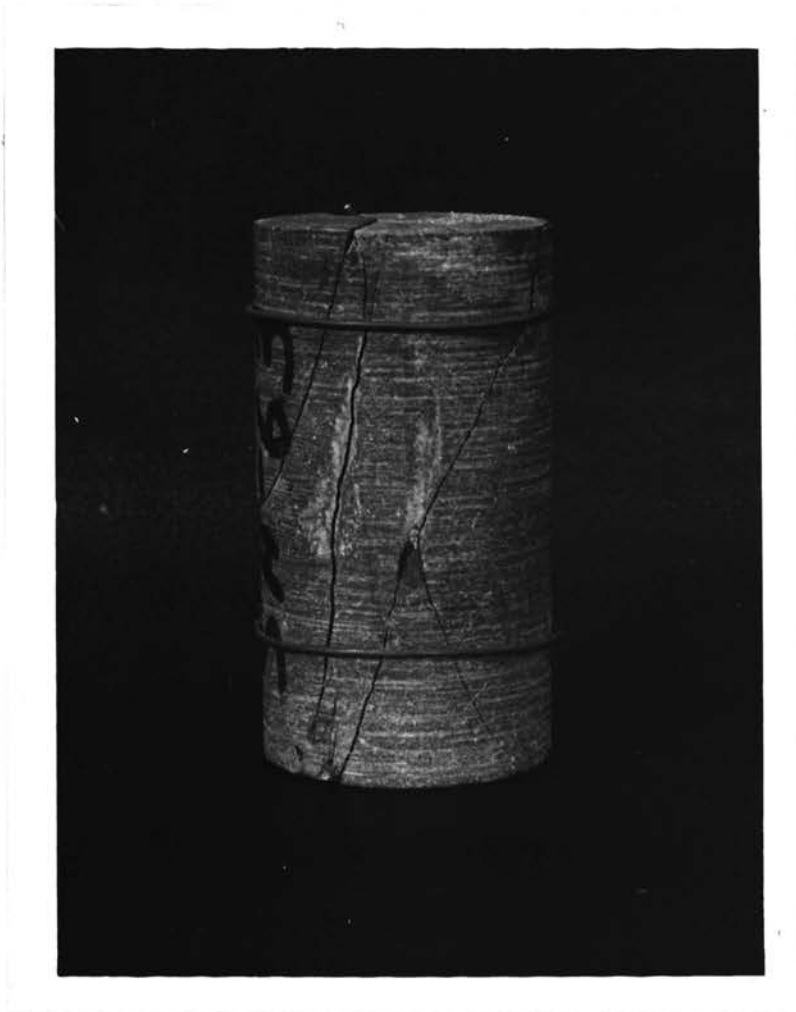
Figure 42 Compressive Failure of a White Pine Shale Sample Under a Condition of 2e, dE-70^\circ .
