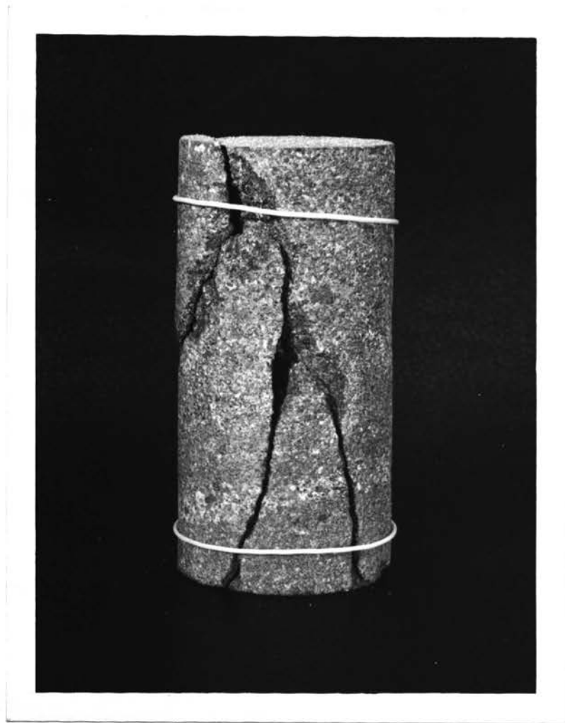
Figure 39 Compressive Failure of a White Pine Sandstone Sample Under a Condition of 3eE-65^\circ
